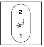
There are two different colors of light that can be selected. Press the upper part of the button for blue light and press the bottom part of the button for amber light. Each light will illuminate the front and rear area of the seat.
